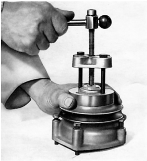
Fig. P.4. Removing the Water Pump Pulley.
