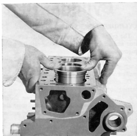
Fig. J.5. Fitting Cylinder Liner.
