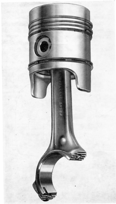
Fig. H.8. Showing Piston Ring Layout.
