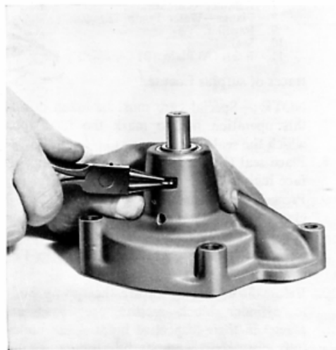
Fig. P.5. Removing Shaft Locating Circlip.
