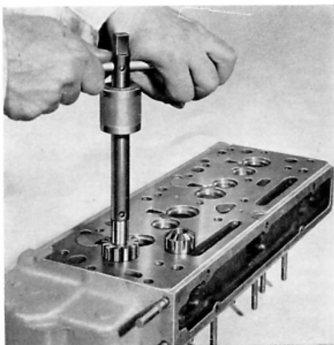
Fig. G.10. Recutting a Valve Seat.
